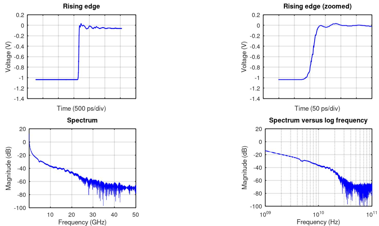
All response chart data collected using pre-production PG-2 pulse generator connected directly to a Tektronix SD-32 50 GHz sampling head attached to a Tektronix 11801C sampling oscilloscope. Spectrum plots are for a single isolated rising edge.
